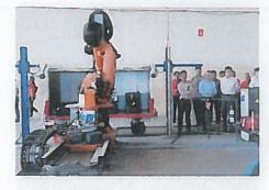
offloader prototype is able to lift a fully loaded baggage trolley, tilt it and offload the entire trolley's load of bags on to the baggage conveyor belt in less than two minutes. This can be achieved by the push of a button.
